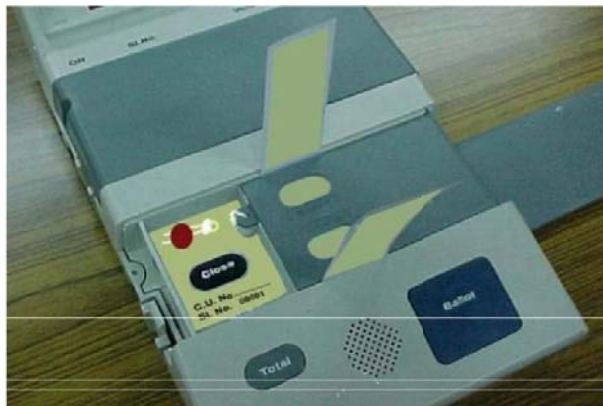
Sealing the inner door with Special Tag
